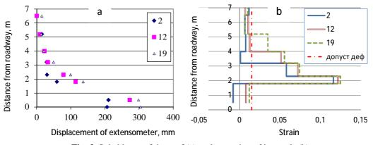
Fig. 3. Subsidence of the roof (a) and extension of intervals (b).
