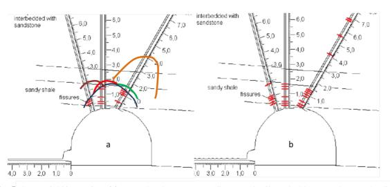
**Fig. 5.** Sequential kinematics of fracture development according to Lubosik et al., 2015: (a), (b) – at the distance 220 m and 12 m in front of the longwall respectively.
