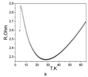
**Fig.1.** Temperature dependence of resistance for n-typeBi<sub>2</sub>Se<sub>3</sub> whiskers with Pd doping concentration of  $1\times10^{19}$  cm<sup>-3</sup> in temperature range: a) 4.2 - 300 K; b) 4.2 - 65 K.
