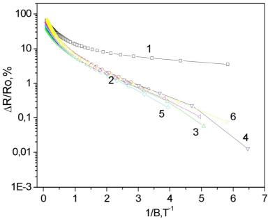
**Fig. 2.** Transverse magnetoresistance of n-typeBi<sub>2</sub>Se<sub>3</sub> whisker at different temperatures: 1 - 4.2 K, 2 - 13 K, 3 - 29 K, 4 - 40 K, 5 - 50 K, 6 - 60 K.
