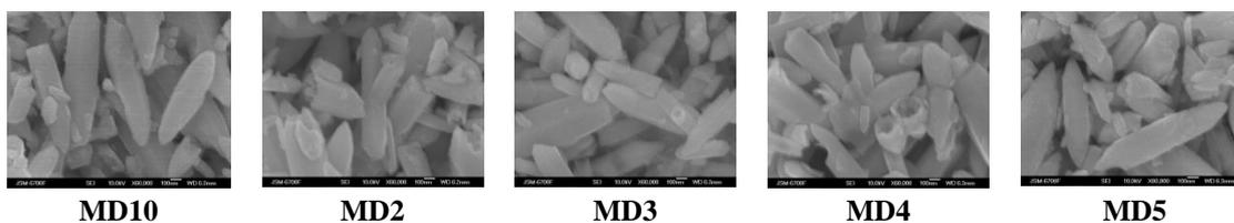
**Fig. 3.** SEM images of samples synthesized at a current density of 0.5 A/cm<sup>2</sup> with a MHB 3000 P2 content of 0.35; 0.4; 0.6; 0.8; 1.0 g/L, respectively.
