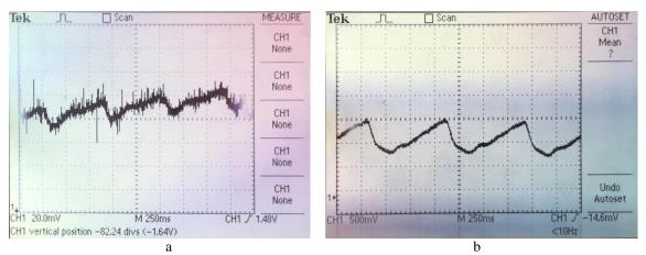
**Fig. 1.** Oscillogram of the signal from the photo-detector after passing light through the finger (a) and the oscillogram after hardware processing and filtering (b).
