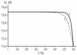
**Fig. 5.** Amplitude-frequency characteristics of the integral signal converters circuit: 1 – amplitude, 2 – phase.
