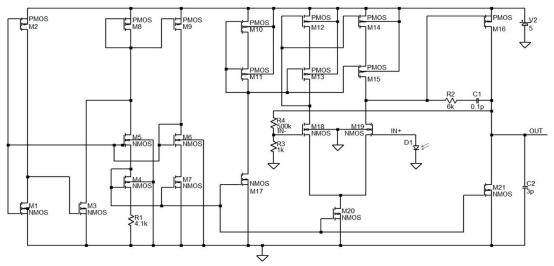
**Fig. 3.** Part of the electrical schematic circuit of the ISC (one operational amplifier) (the dimensions of the *p*- and *n*-channel MOS transistors are given in Table 1).
