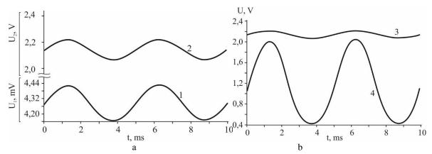
**Fig. 4.** Timing diagrams of the simulation of the functioning of the ISC in LT SPICE: a – amplification of the output signal of the photo-receiver, b – compensation of the constant component, filtering and amplification of the useful signal over the entire dynamic range of the ADC. 1 – input signal, 2 - SENS1 output, 3 - SENS2 output.
