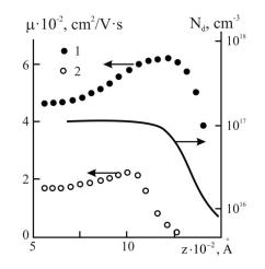
Fig. 1. Profiles of mobility and concentration of electrons for structures with homogeneous doping for GaAs-layers at different temperatures: 1 – 77 K; 2 – 300 K
