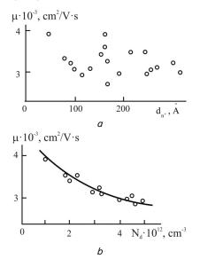
Fig. 2. Dependence of the electron mobility on the thickness of deepened layer (a) and the product of concentration on the thickness of the deepened layer (b) for GaAs epitaxial layers
