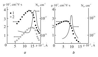
Fig. 3. Profile of mobility and concentration of electrons at different temperatures (1–77 K, 2-300 K): a - structures with deepened n-GaAs-layer; b - structures with  $\delta$ -layer
