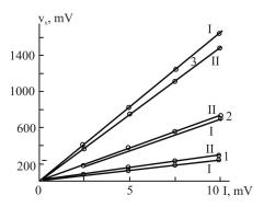
Fig. 6. Hall voltage as a function of control current for both I and II types of hallotrons
