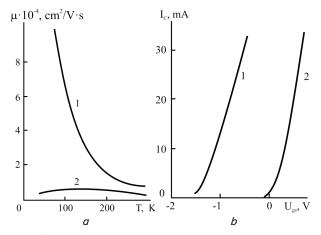
Fig. 9. Temperature dependence of electron mobility for 2DEG-layer (*a*) and drain-gate characteristics of ShFT (*b*): normally open (1) and normally closed (2)
