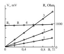
Fig. 5. The Hall voltage for three values of the control current (2.5, 5, and 10 mA – curves 1, 2, 3, respectively) and resistance (curve 4) as a function of magnetic induction
