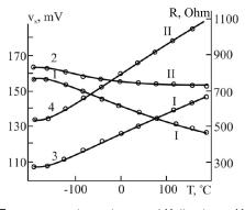
Fig. 7. Temperature dependences of Hall voltage (1, 2) and resistance (3, 4) for both I and II types of hallotrons
