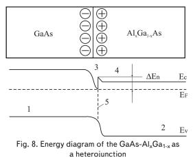
The electrons, accumulated in region 3, are located in a potential well and can move in weak electric fields only along the interface 5 in the plane perpendicular to the plane of Fig. 8. Therefore, such a set of electrons in the region 3 is called a two-dimensional electron gas (2DEG), thus emphasizing that in the weak fields these electrons cannot move in the third dimension.
