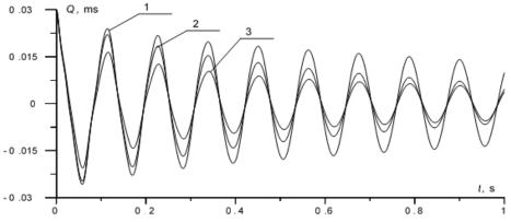
Figure 2: Transient motions of the tube central component (h = 0,001m): 1 is the first experiment, 2 is the second experiment, 3 is the third experiment
